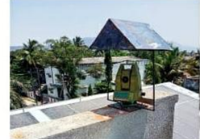
Total Station for measuring settlements and deformations.
