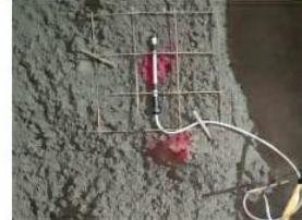
Strain gauges capture deformation or elongation. They are attached with wires to monitor the deformation in shafts.
